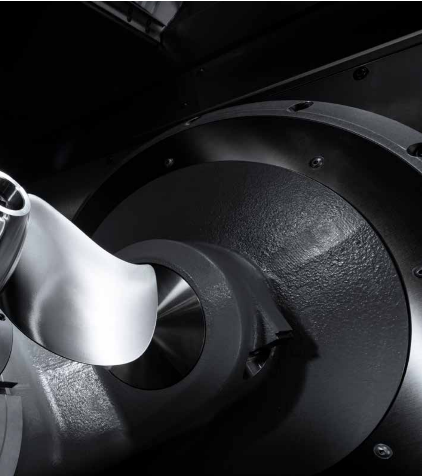
HERMLE C 42 U dynamic in 5-axis version | Machining of a propeller for the sports and leisure industry.
