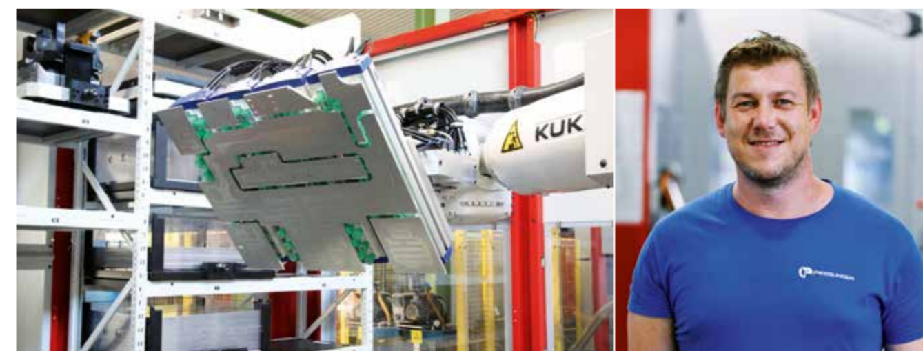
left The robot can both transfer circuit boards, pallets or individual components to the C 42 and remove them. That way the cell can be used in an ultra-flexible way. right Roland Berger, Production Manager from Piesslinger
